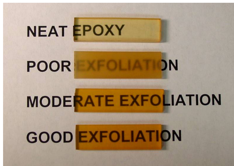
Fig. 5.5. Images of neat epoxy and epoxy/ \alpha -ZrP nanocomposites with different levels of exfoliation.
