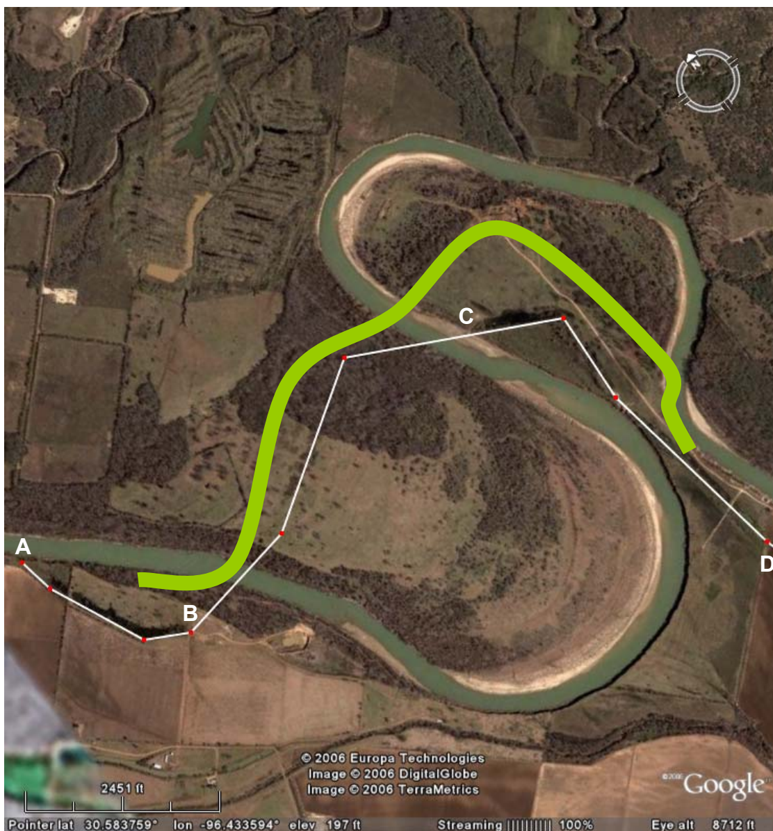
Figure 6.6. Levee Breach at Mile 9. This is the largest of the Burleson levee breaches. The wide light green line represents the approximate channel of the river in 1910. The thin white line is the estimated location of the original levee. Both are taken from Nagle's 1911 map in Plate 1. The levee is still in place today from point A to point B and from C to D. The dark area lining the northern side of the trace of the levee between A and B and to the right of C is the borrow pit. Between B and C, the levee has been completely washed away by the river meander which has advanced to the right (southeast) almost a mile since the levee was first constructed in 1910. Satellite image is from Google Earth.
