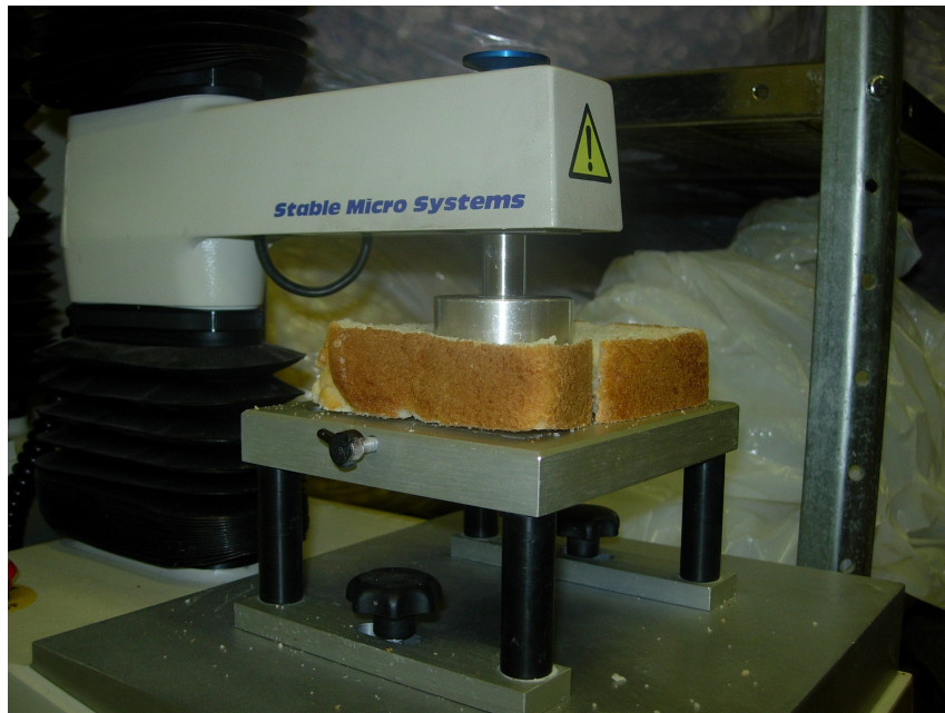
Fig. 6. Use of the Texture Analyzer to determine crumb firmness.
