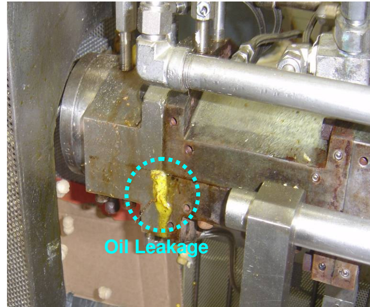
Fig. 5. Visible oil leakage on external of extruder head barrel A) No external oil B) Exterior oil
