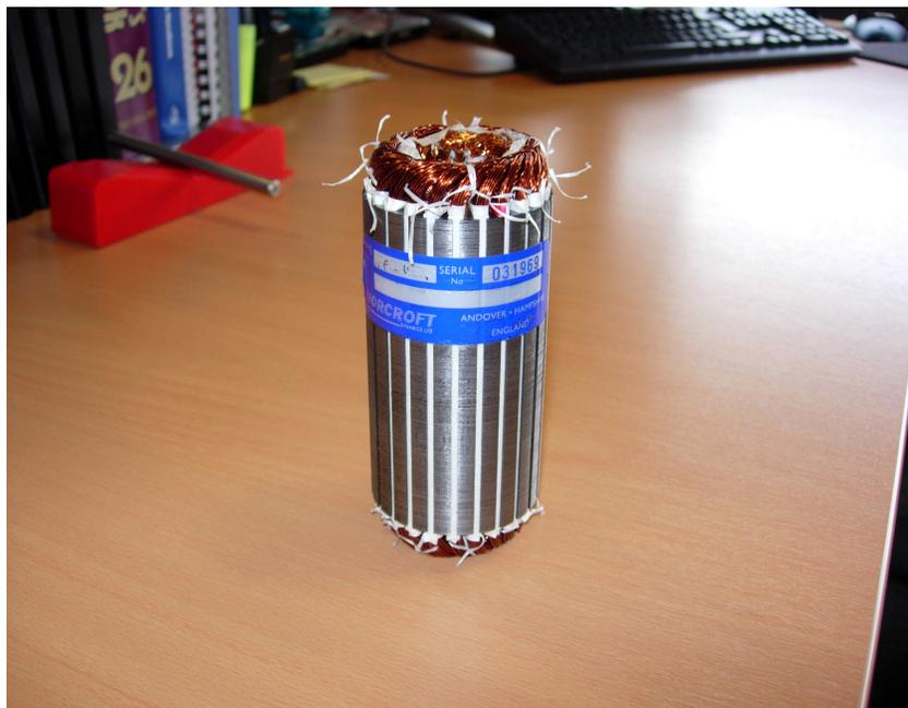
Fig. 3.26. Prototype dual winding stator.
