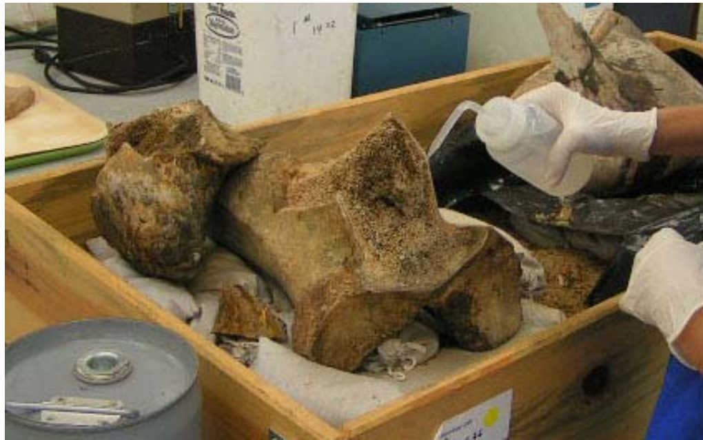
Figure 4.2. Showing the methodology of conserving the Columbian mammoth using methyltrimethoxysilane (photography by Robert Larsen).
