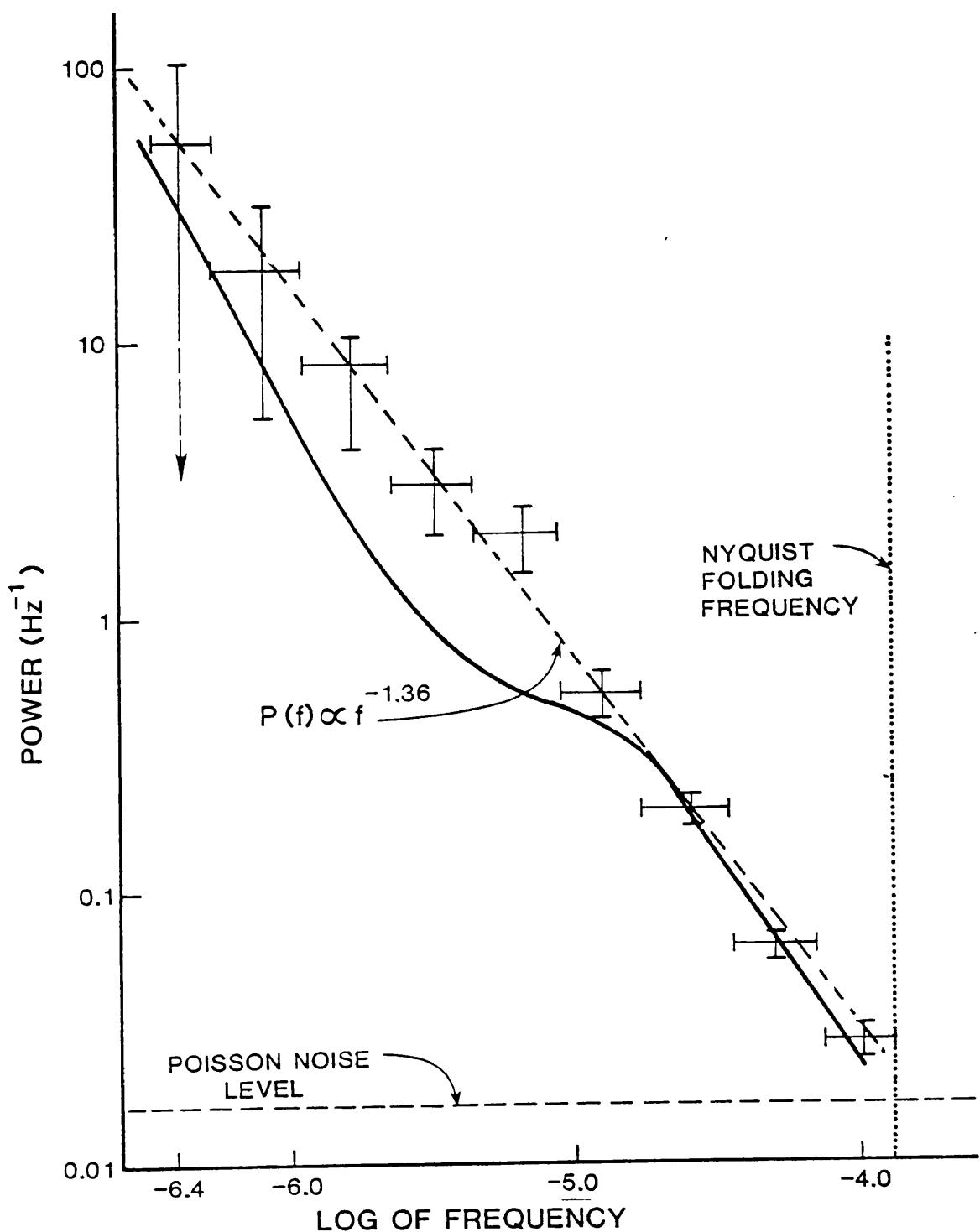
**Fig. 16.** A comparison of the muon PSDF at TAMU with the theory using data by Quenby and Sear. Frequency is in Hz.
