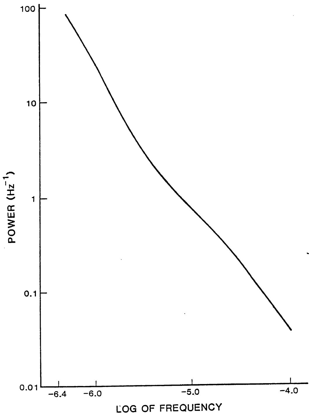
**Fig. 5. Predicted PSDF for a purely equatorial telescope.**
