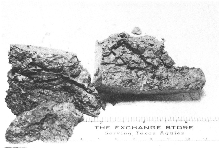
a. The Fissures in Beaumont Clay
