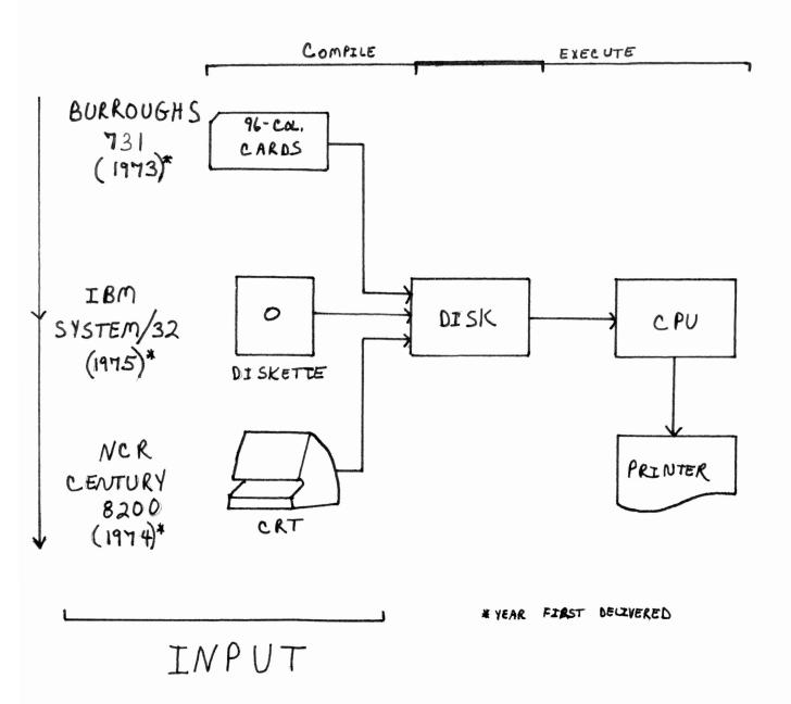
Figure 7. Diagram of Input Device of Each Computer System.
