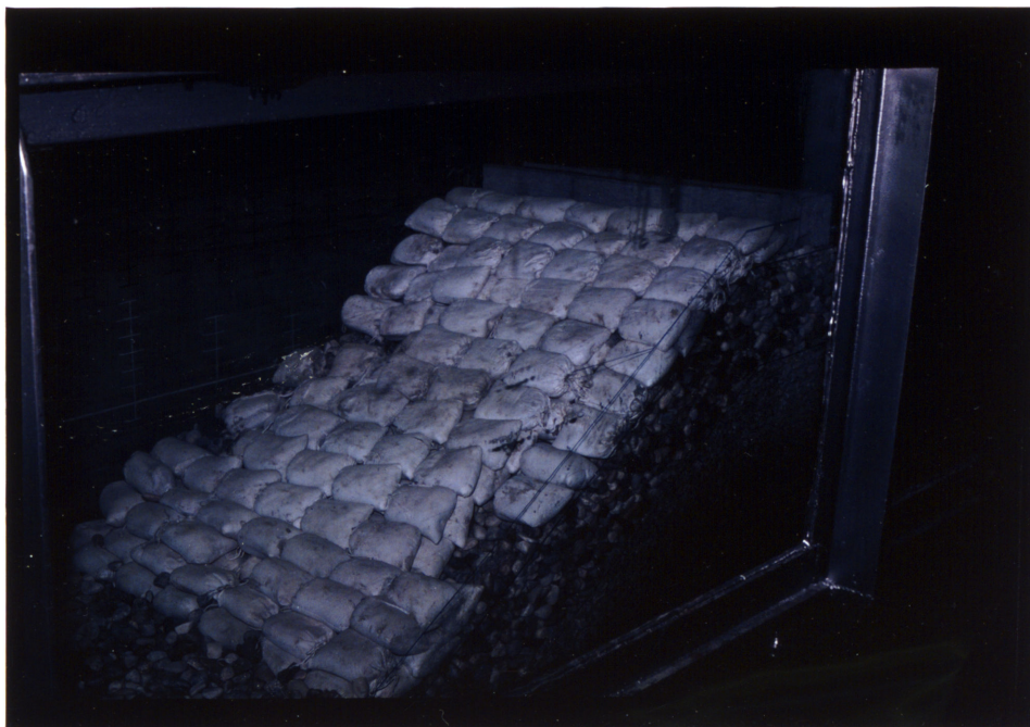
Fig. 8. Breakwater After Completion of Testing
