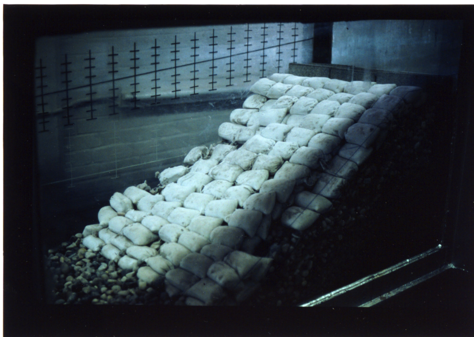
Fig. 9. Breakwater After Completion of Testing
