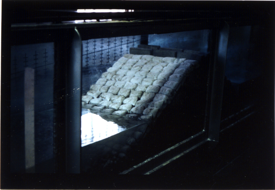
Fig. 6. Breakwater Prior to Testing
