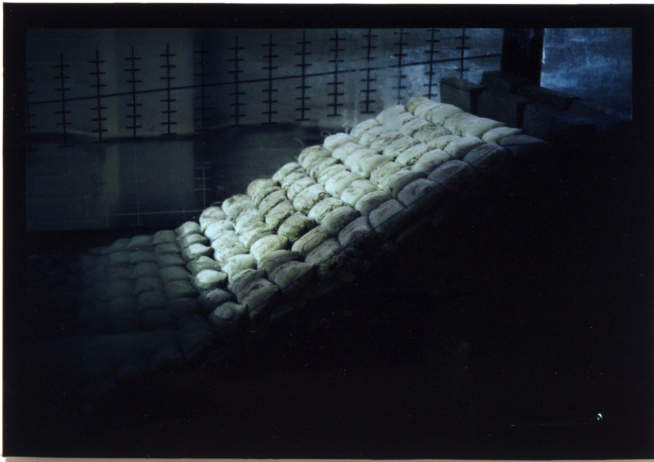
Fig. 7. Breakwater Prior to Testing
