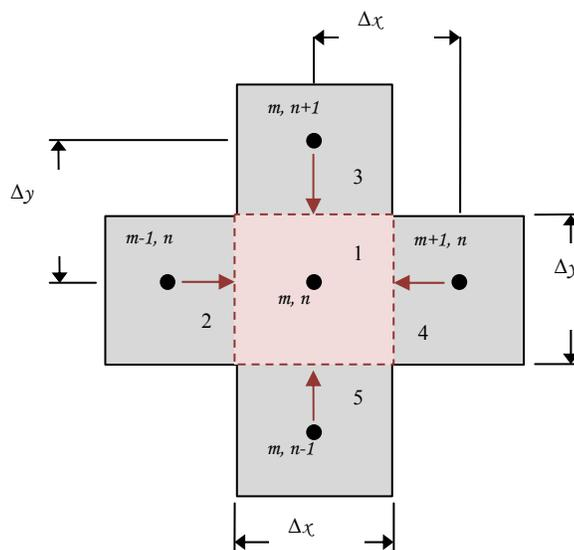
**Fig. 2.1.** Conduction of adjoining nodes to the reference node. <sup>1)</sup>
