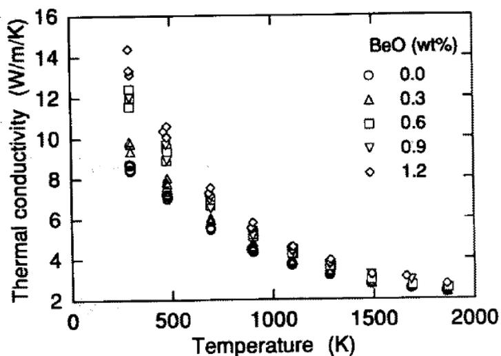
Fig 2.2. Thermal conductivity of BeO infused pellets. <sup>2)</sup>
