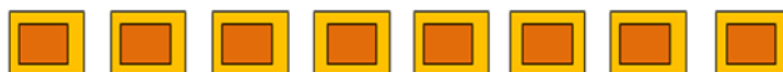
Figure 12. Schematic of the 50 nm frames lithography script, 1x8 section of the 8x8 array.
