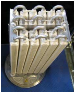
Figure 2: Coated finned-tube adsorber heat exchanger
