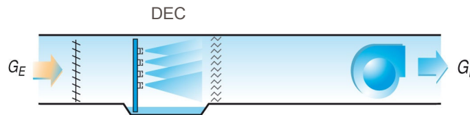
Figure 3. AHU at Peñagrande station, Madrid, with DEC (diagram)
