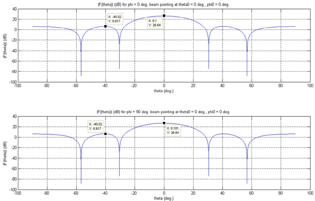
Figure 1: Array Factor 9dB) for a 5x5 array with amplitude tapering for  $\Phi=0$  and  $90^\circ$  respectively.
