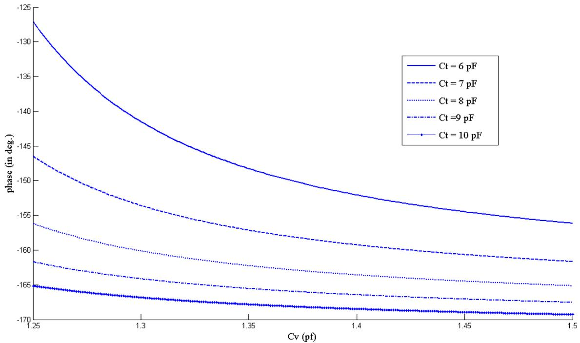
**Figure 4: Phase shift (in deg.) vs.  $C_v$  (pF) for different values of  $C_t$ .**
