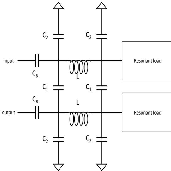
**Figure 2: RTPS with identical resonant loads**
