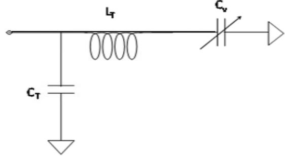
**Figure 3: Resonant load with L-match impedance transformation.**
