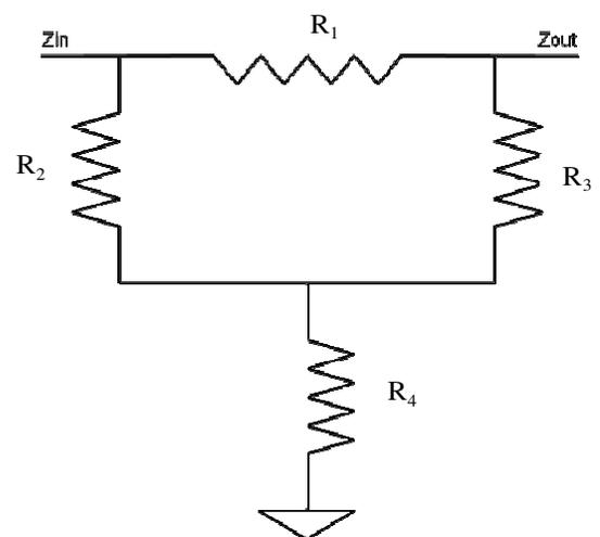
**Figure 5: Basic bridged-T attenuator**
