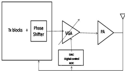
**Figure 6: Complete block diagram with VGA and RTPS for the Tx chain for a single array element**
