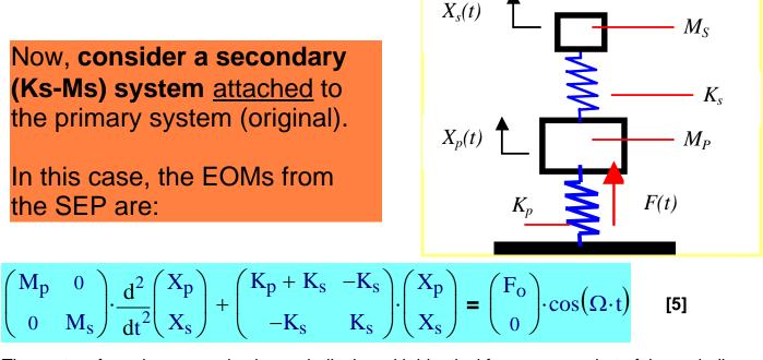
The system forced response is also periodic, i.e. with identical frequency as that of the periodic excitation force. Thus, let **The combined system is**
