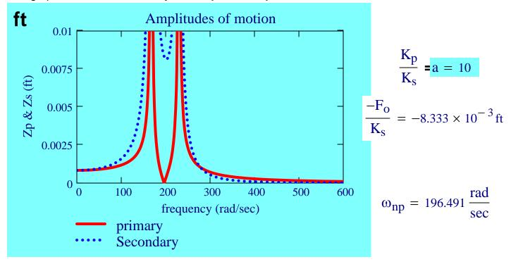
Note the amplitude of motion is zero for the primary system when excited at its original natural frequency. The secondary system does have a large amplitude of motion and is out of phase 180 degrees with the excitation force.
