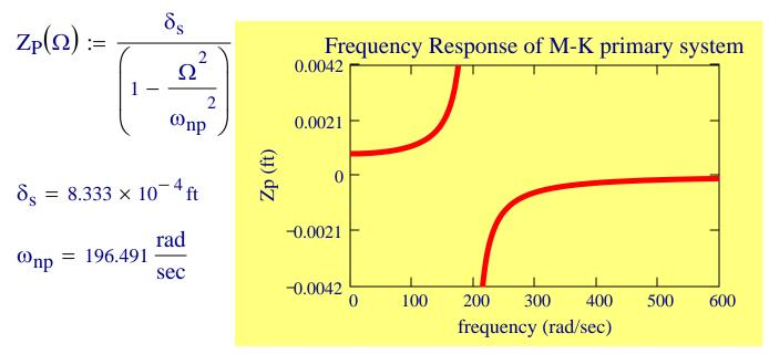
Note the very large amplitude of motions (unbounded) for excitation at the system natural frequency. In the graph above, Zp>0 means in phase with the external force, Zp<0 means 180 deg out of phase with external periodic force.
