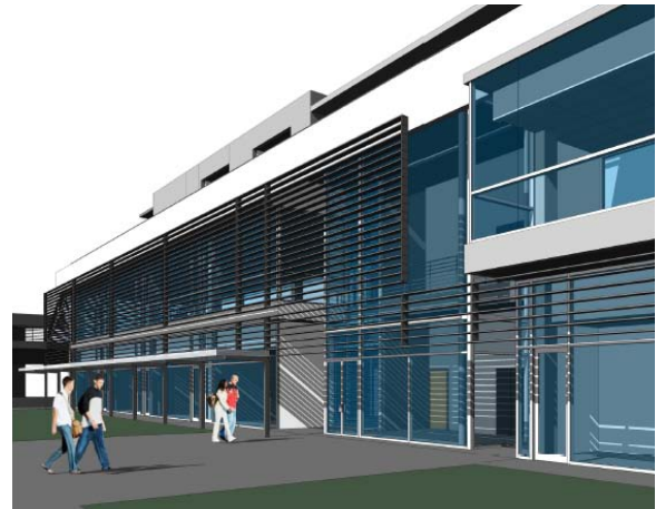
Figure 1. Building #1 Initial Exterior Shading Design
