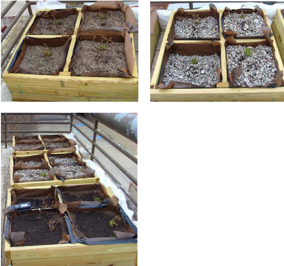
Fig. 6 –Completed green roof plots. Clockwise from top left: completed box of shale with compost; completed box of recycled concrete and compost; and all completed boxes with the box of topsoil and compost in foreground.
