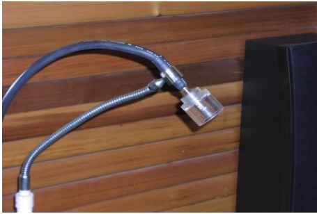
Fig. 13 Attach cap at the emission part after repairing
