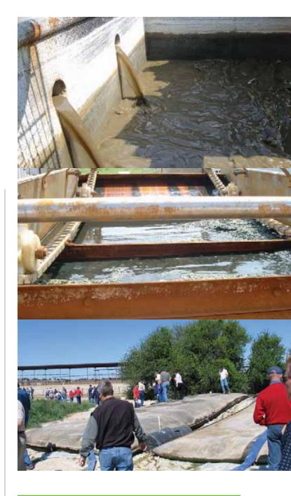
(Top) In the first stage of the electrocoagulation process, dairy effluent enters the mixing tank and lime, coagulants and an emulsion polymer are added and agitated.
