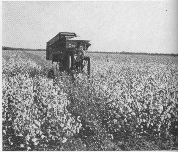
Fig. 35. Large-to-medium size cotton on heavier, river bottom soils is machine harvested more efficiently with a spindle picker in open-boll types.
