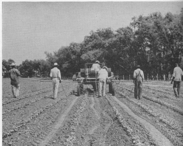
Fig. 22. A regular insect control spray rig can be adapted for a crew of four to spot-spray grass in cotton.
