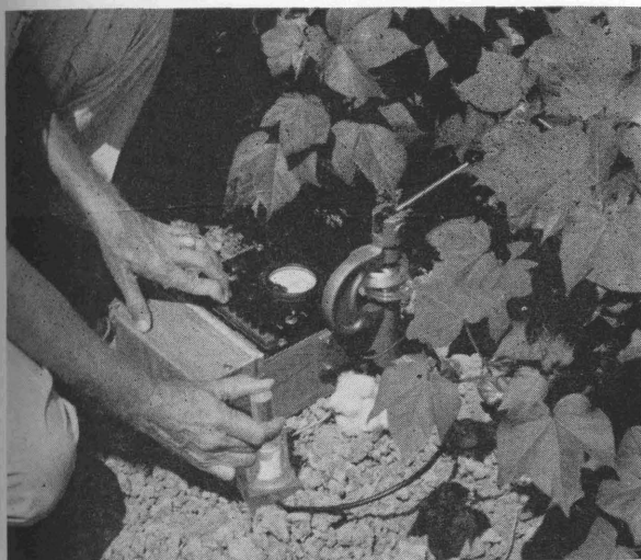
Fig. 37. A moisture meter can be used in the field to determine moisture content of seed cotton.
