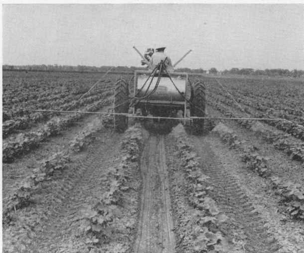
Fig. 24. One nozzle per row will give good coverage.
