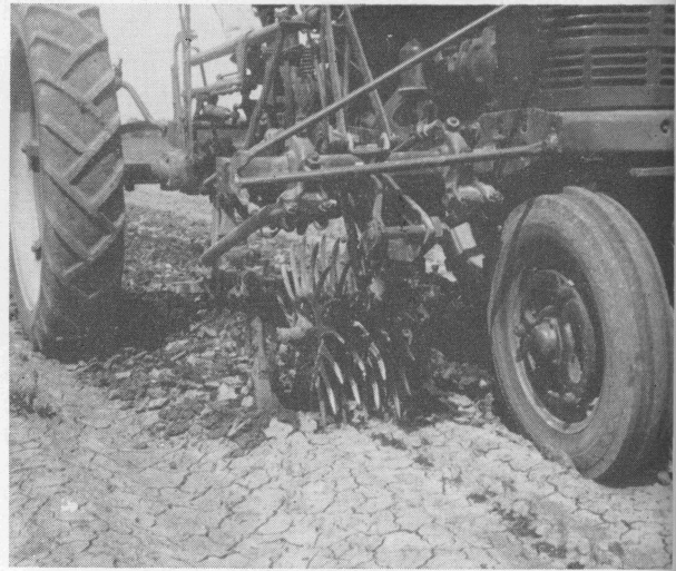
Fig. 13. Cultivator mounted rotary hoe "floats" inside the front sweeps. Sweeps should be new type, low crown, broad, low wings for high-speed cultivation without heavy "dirting."
