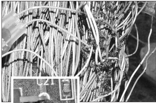
Accumulations in electrical equipment cause short circuits and equipment failure.
