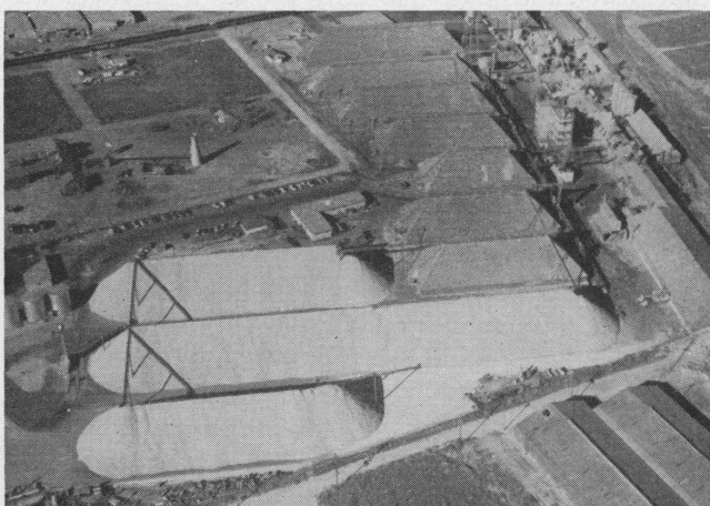
Some 212,000 tons of cottonseed are stored in pyramids on the ground at this Lubbock cotton oil mill.
