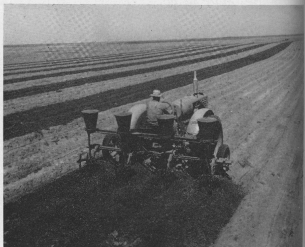
A lister type planter planting four rows of cotton at a time on the High Plains.
