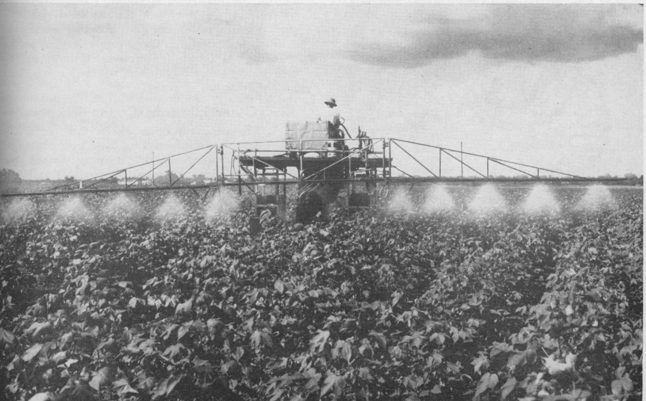
Covering 14 rows each trip across the field makes short work of ground spraying to control cotton insects on experimental farms near College Station.
