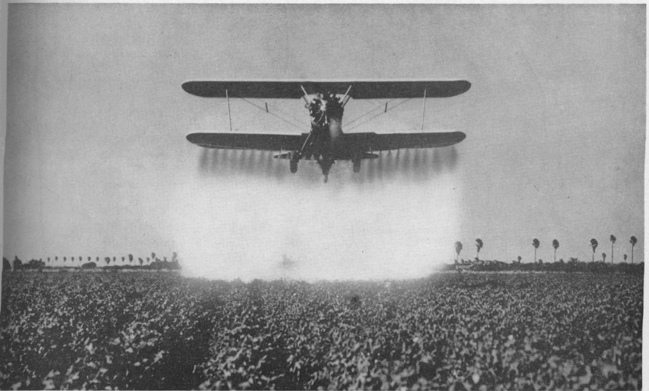
Late season airplane spraying in the Lower Rio Grande Valley to control cotton insects. Such planes can spray about 20 acres on one load. The airplane also is used to apply defoliants and desiccants.
