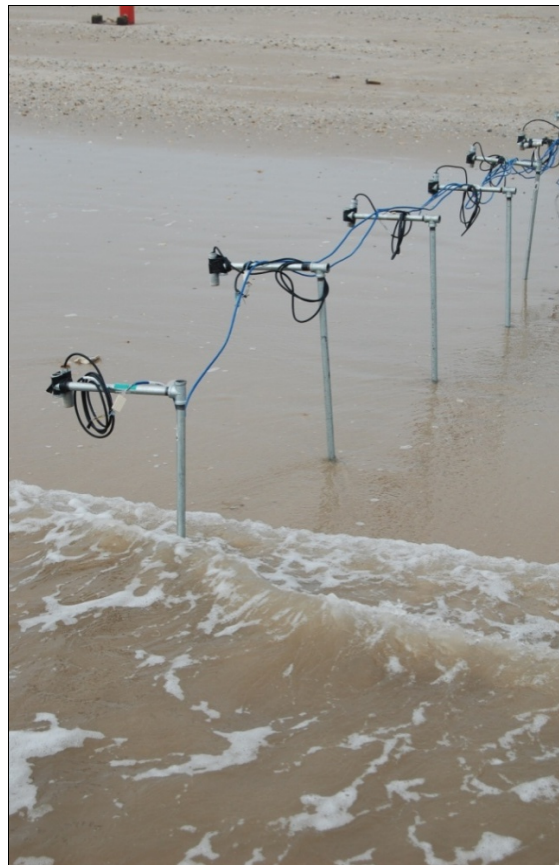
Figure 3. Matagorda field site set-up for ultrasonic sensors on cross-shore transects.
