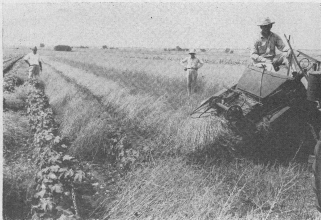
Figure 15. Windrowing Hubam clover with a converted grain binder.
