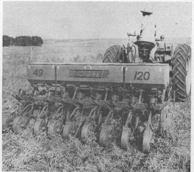
Figure 46. Deep-furrow, hard-ground drill that is doing a good job of putting small grain and fertilizer 3 to 4 inches deep into hard, dry ground. This drill, with shoe-type openers and spring shanks, is useful for drilling into biennial clover, established grass, lanes or heavy residues of any kind.
