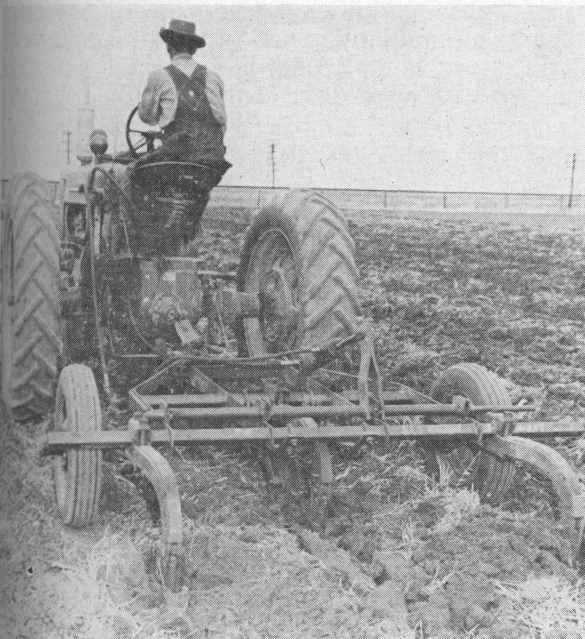
Figure 44. Subsurface or trash-mulch plowing is a promising new practice for economy, efficiency and conservation in the Blackland.
