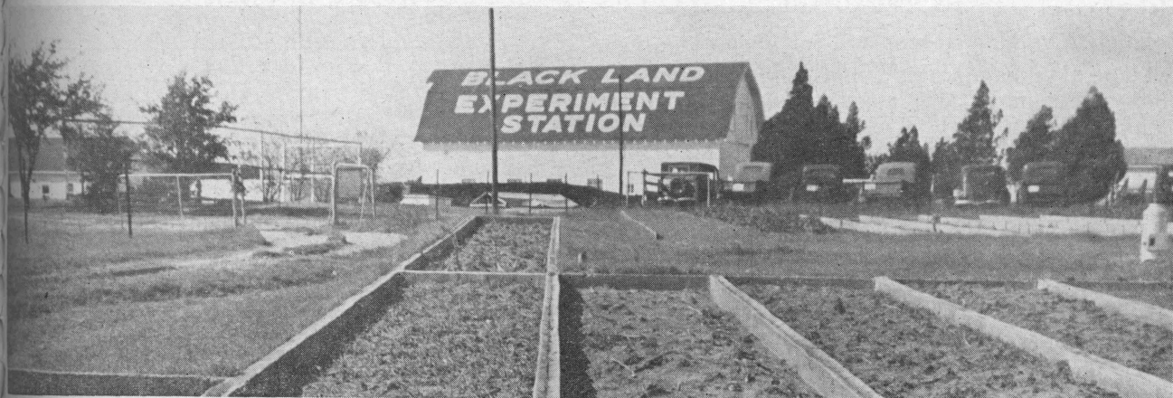
Figure 9. Runoff-erosion plots on 4 percent slopes. Plot 3, continuous corn, shows a sealed-over surface compared with Plot 2, where Hubam stubble has been spaded. The soil level in Plot 3 is about 3 inches lower because of heavy erosion losses during 20 years.
