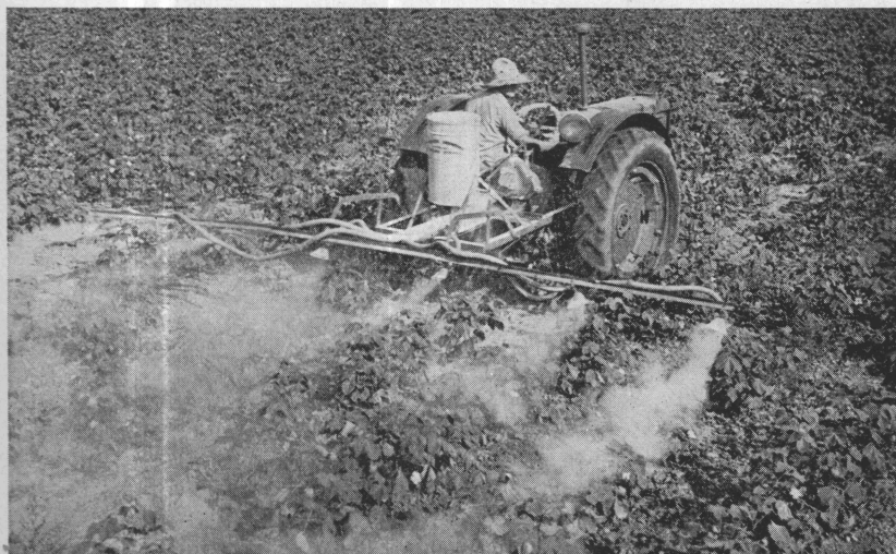
Figure 35—Dusting cotton with a tractor-mounted duster. The mechanism of the duster is driven by the power-take-off of the tractor. It may also be driven by an auxiliary gasoline engine mounted near the hopper.
