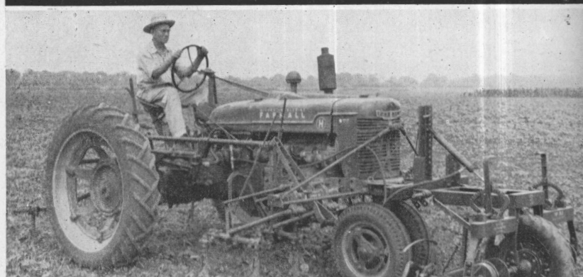
Figure 24—Two-row tractor equipped with two-row front-mounted mechanical cotton chopper, two-row cultivator and rotary hoe attachments between the front sweeps of the cultivator.
