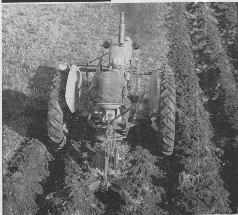
Figure 9—Front view of front-mounted or push-type middle-breaker or lister.
