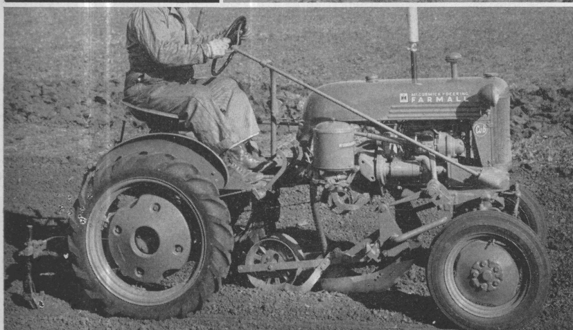
Figure 16—A single-row planter mounted on a small tractor. Note the runner seed furrow opener and the press wheel cover. A scrapper coverer throws extra soil over seed between furrow opener and press wheel.
