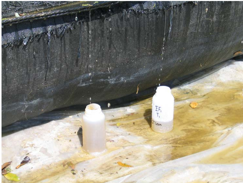
Fig. 6. Effluent Being Sampled from a Dewatering Geotube®
