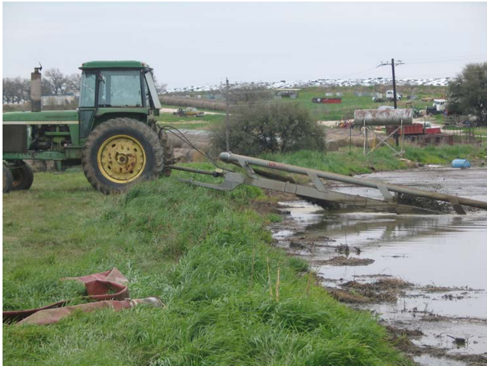
Fig. 3. PTO Driven Chopper Pump in the Primary Lagoon
