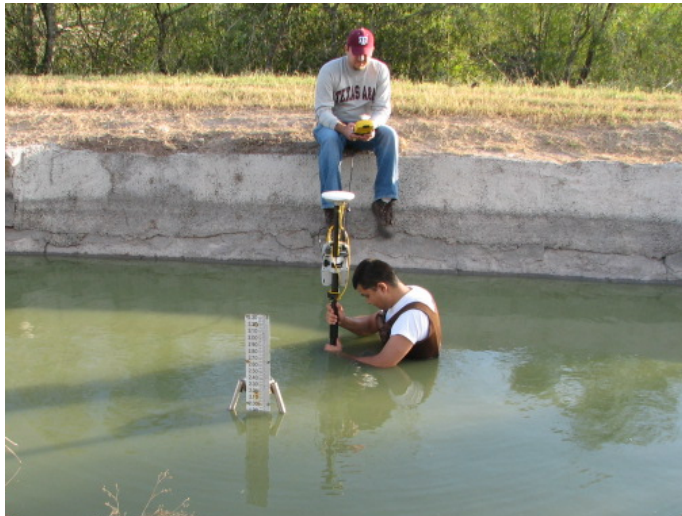
Figure 3. Shows the GPS survey and a staff gage
