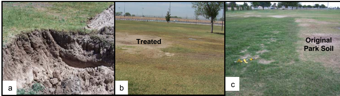
Fig. 13 Effects of profile modification of Sanlei silty clay at Shawver Park, West: Stratified profile (a), after inverting (b), and by May of 2007.
