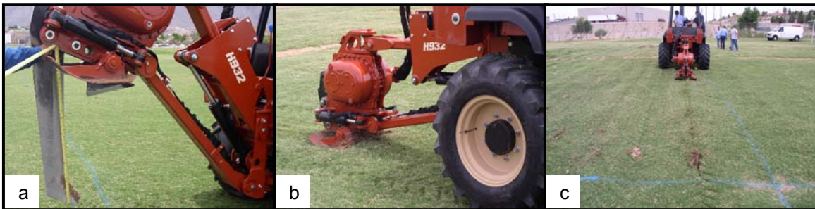
Fig. 21 A vibratory chisel used at the Galatazan Park.
