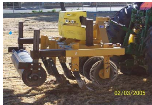
Fig. 10 Modifications made by Mr. Sam Calhoun to the initial chiseling unit: packing roller and weight bars.
