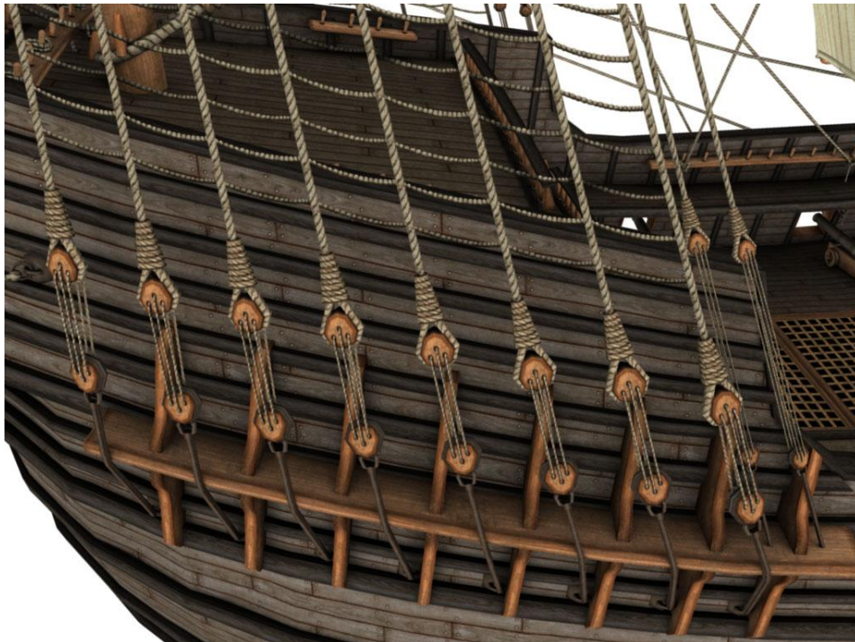
Fig. 24. Deadeyes fastening shrouds and backstays
