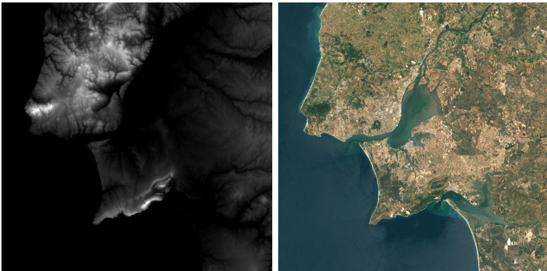
Fig. 52. Terrain height map (generated from SRTM data) and color map (generated from Landsat data)
