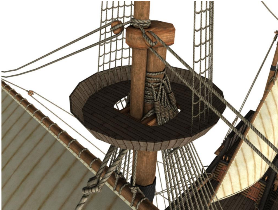
Fig. 25. Shrouds and mainstay tied off at top of the main mast
