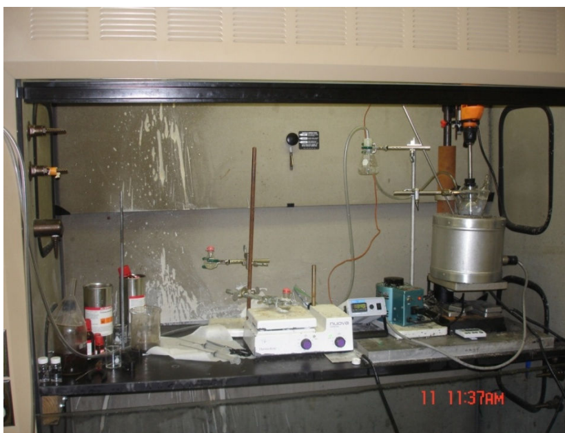
Figure 4. Experimental set up to fabricate quantum dots.
