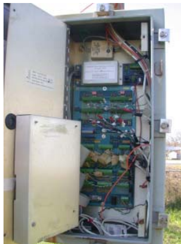
Figure 176: Data logger (Synergistic Data Logger C180E) (Source: Kim 2006)
