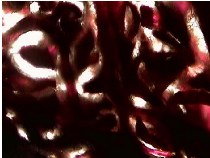
FIGURE 11. Air Dried leather under bright field microscopy. Note the dark appearance and total separation of fibers from each other.
