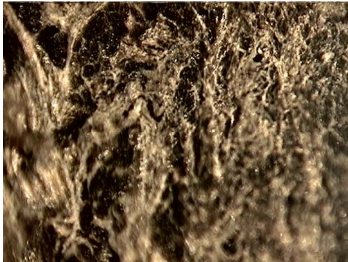
FIGURE 14. Leather treated to 30% with sucrose. Note grainy texture, in which some individual sugar crystals can be discerned.
