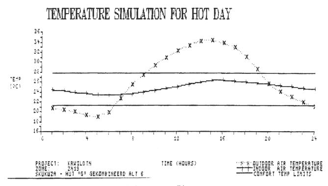
Figure 11. Underground air pipe, ceiling fan for summer conditions
