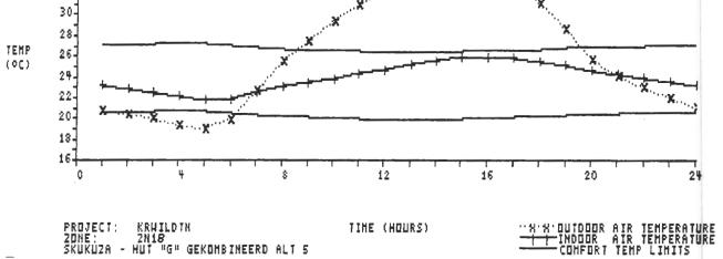
Figure 9. Cavity filled with 50mm polystyrene plus 80% direct evaporative cooling for summer conditions
