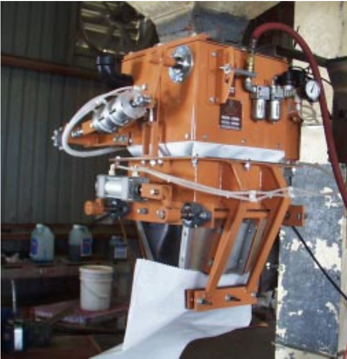
Bagging machine used to package innoculated soybeans for Helena Chemical Company, a profitable sideline with very little additional investment.
