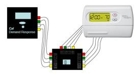
Figure 3: Wireless HVAC actuator and thermostat interface.
