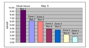
Figure 11: Day 3 comparison of the furnace and fan energy required to heat zones 1-4 compared to the energy required to heat the whole house.
