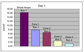
Figure 9: Day 1 comparison of furnace and fan energy required to heat zones 1-4 to the energy to heat the whole house.
