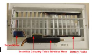
Figure 4: Vent louver design with Tmote controlling Servo, both the Tmote and Servo are powered from separate battery packs.
