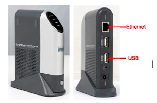
Figure 2: NSLU2 used as the server-controller unit. On the left side is a front view of the device. Two USB ports and one Ethernet port are shown on the right side.
