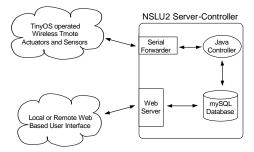
Figure 6: Server-client software system architecture.
