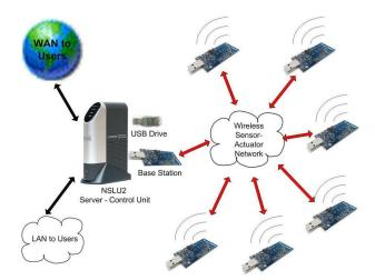
Figure 5: Embedded server - embedded wireless client - internet based client architecture.
