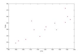
Figure 7: Power (Watts) as function of Vent Flow (CFM) data for various test configurations. \_The power versus flow data suggests that fan power increases as vent flow increases.
