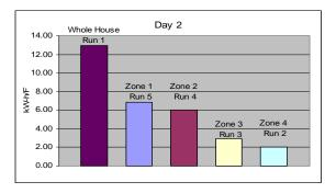
Figure 10: Day 2 comparison of furnace and fan energy required to heat zones 1-4 compared to the energy required to heat the whole house.
