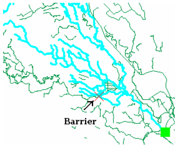
Figure 5.7: Placing a Barrier to restrict tracing
