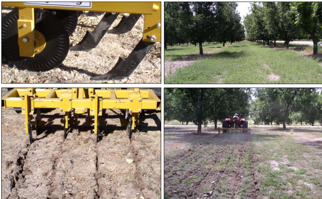
Fig. 4. A minimum-till surface chisel being tested for alleviating soil surface compaction in pecan orchards.
