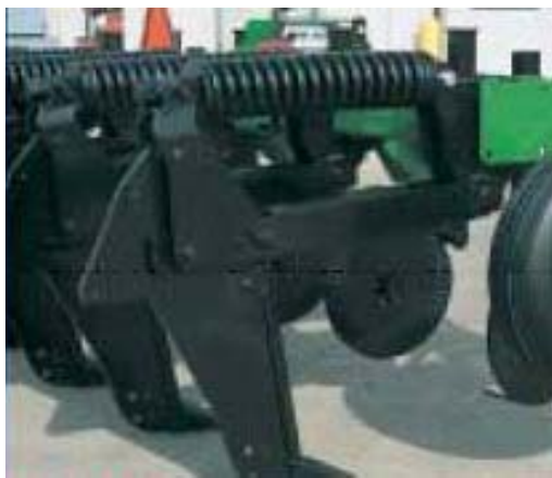
Fig. 5. Spring-loaded subsoiling shank penetrating 70 cm deep.
