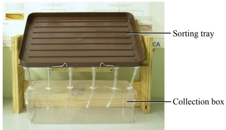
Fig. 3. Sorting tray and collection box used for separating termites from trap debris.
