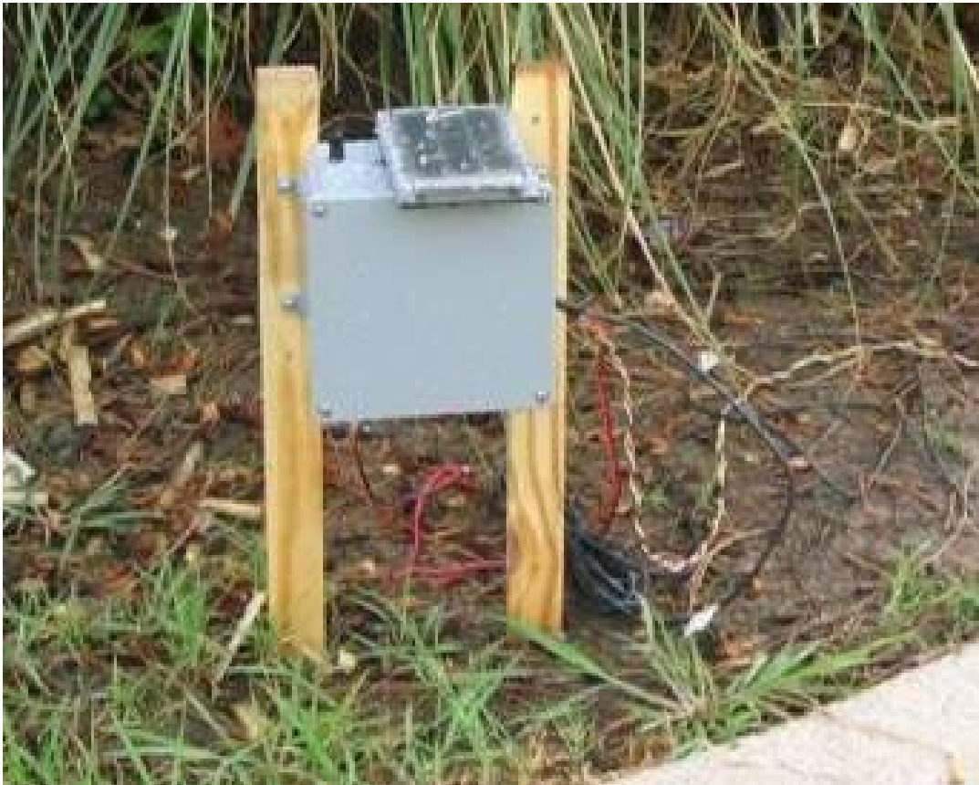
Figure 16. Field deployment of wireless soil monitoring node.
