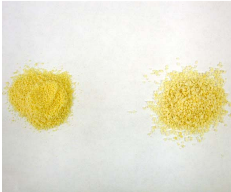
Figure 3. A comparison of 0.025% Advion™ with small sized grit (<1 mm/granule, pictured on the left) and 0.025% Advion™ with standard sized grit (~2 mm/granule).
