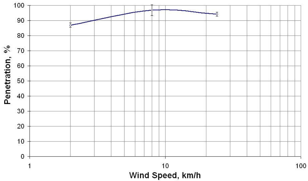
Figure 17: BSI-100, penetration as a function of wind speed. Particle size: 10.1 μm AD.
