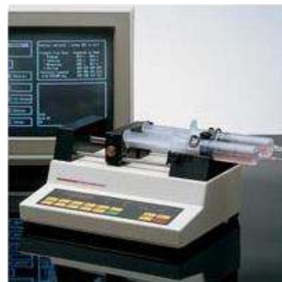
Figure 3. The original Harvard Apparatus media pump could only handle three 60 mL syringes at once.
