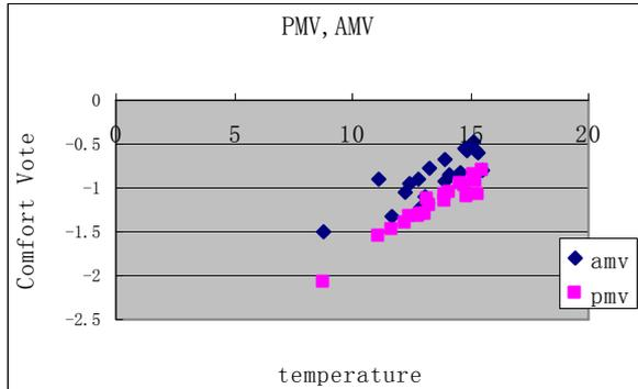
**Fig. 2 PMV, AMV vary with indoor air temperature**
