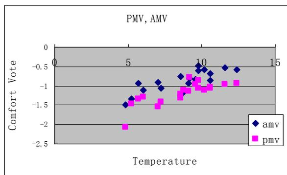
**Fig.4 PMV, AMV vary with outdoor air temperature**
