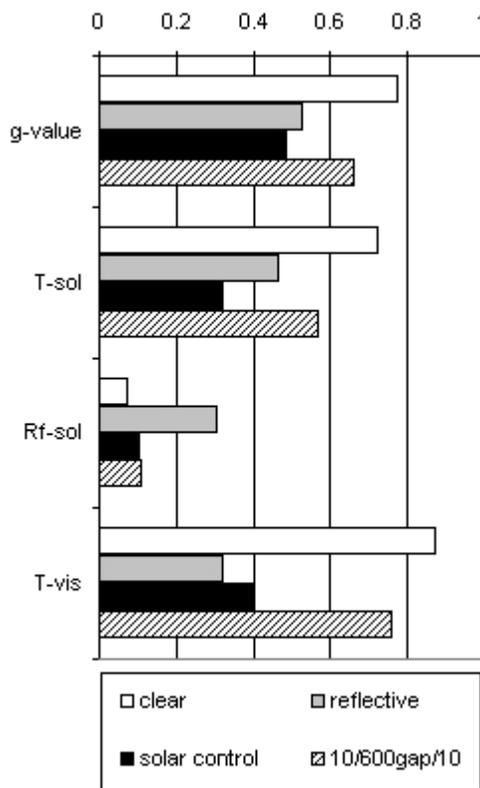
**Figure 5. Glazing properties of glazing types used**
