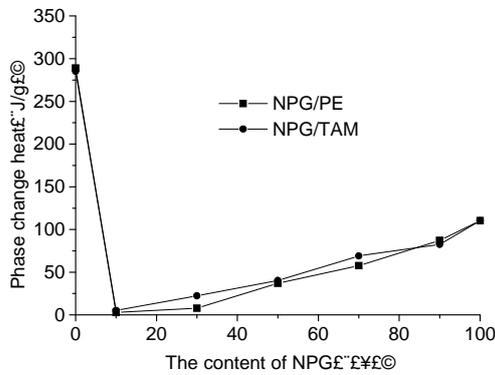
**Fig. 2** The relationship between phase change latent heat and constituent of binary systems NPG/PE and NPG/TAM
