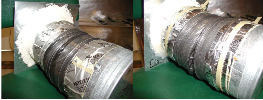
Figure 9. (Left) Shrinkage and Delamination Among the Unclamped Specimens (Showing Here Result of 5 Months of Aging), and (Right) Oozing of the Adhesive Layer in the Foil-Butyl Tape (Tape 4) Specimens (Showing Result of 5 Months of Aging)
