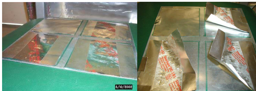
Figure 7. A Baking Specimen Following the UL 181B Temperature Test Protocol Consisting of Three Samples of Tape (Tape 3) and One Control Sample of the Substrate (Aluminum Foil) Before Testing and After Four Weeks of Testing
