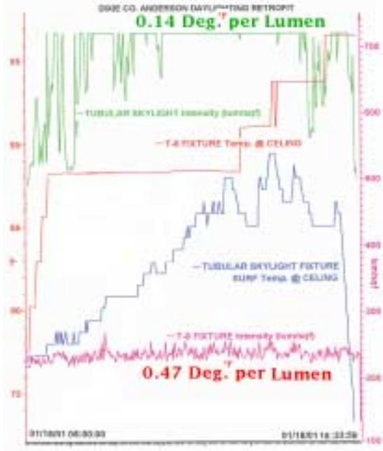
Reference Figure 3 shows the heat gain in a Gymnasium when the standard Metal Halide lighting system **is turned on** with a electrical load of 28 Watts per lumen, you will note that at playing level ( 5 feet from the floor ) the temperature increases better than 2.6 deg. F in 6 minutes. Though not represented on the chart, the increase in foot candles when we
