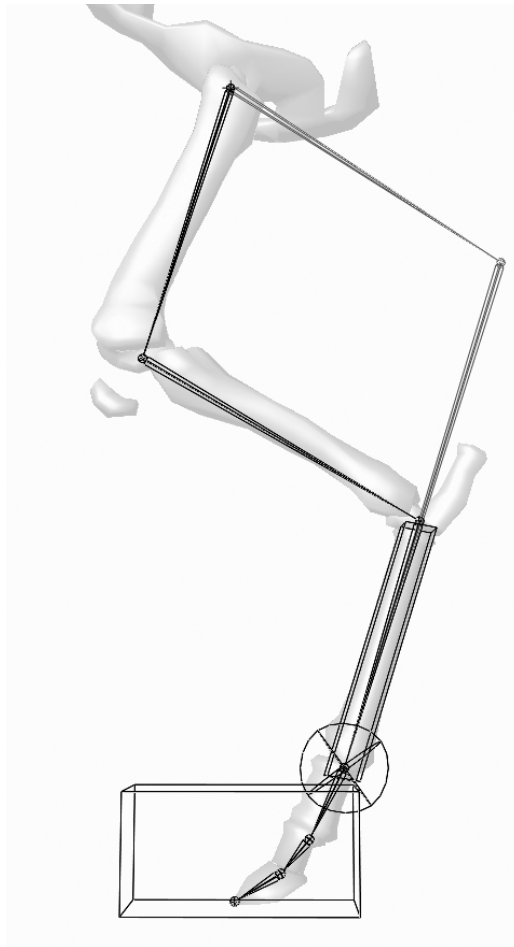
Figure 21: Reverse leg structure used to generate reciprocal motion in stifle and hock joints.
